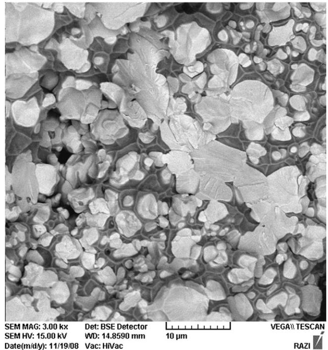
Fig. 9. Typical BS-SEM micrograph of a fracture surface of infiltrated specimen after compression at 663 MPa and sintering at 1550 °C for 4 h.
