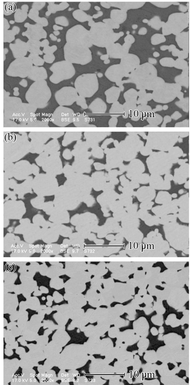
Fig. 6. BS-SEM micrographs of infiltrated tungsten specimens after sintering at 1550 °C for 4 hours compressed at: (a) 245 MPa, (b) 491 MPa and (c) 663 MPa.
