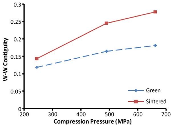
Fig. 7. W-W contiguity change vs. compression pressure for green and sintered specimens.
