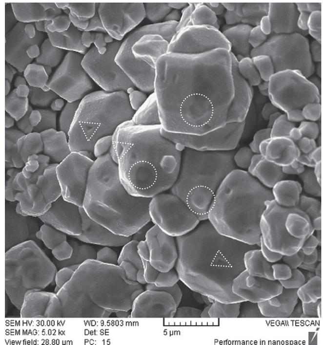
Fig. 4. SE-SEM micrograph of fracture surface of specimen compacted at 663 MPa; circle: example of tips flattening, triangle: example of tips penetrations.
