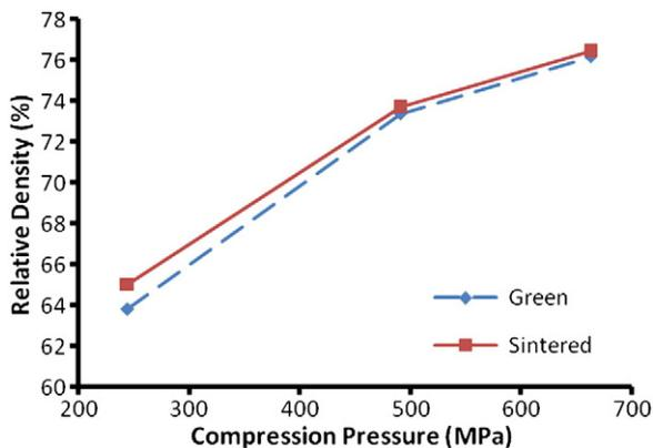
Fig. 8. Density vs. compression pressure for green and sintered specimens.
