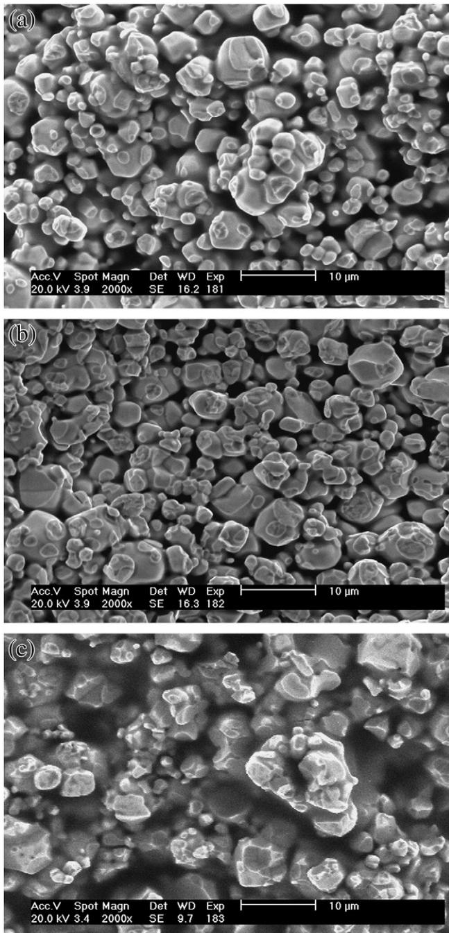
Fig. 5. SE-SEM micrographs of fracture surface of specimens compacted at (a) 245 MPa, (b) 491 MPa and (c) 663 MPa and sintered at 1550 °C.
