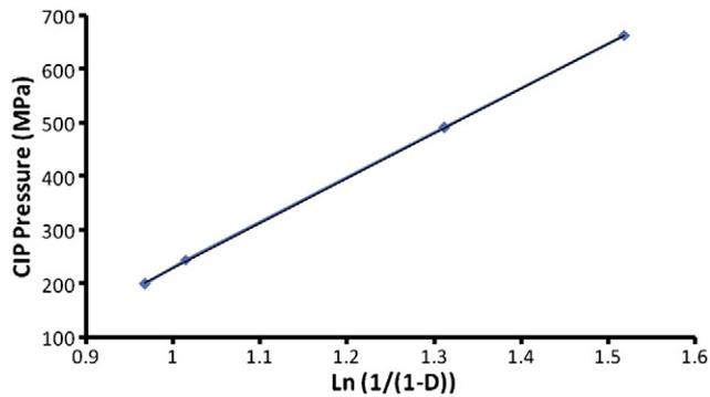
Fig. 2. Pressure of CIP compaction vs green density of the compacts.
