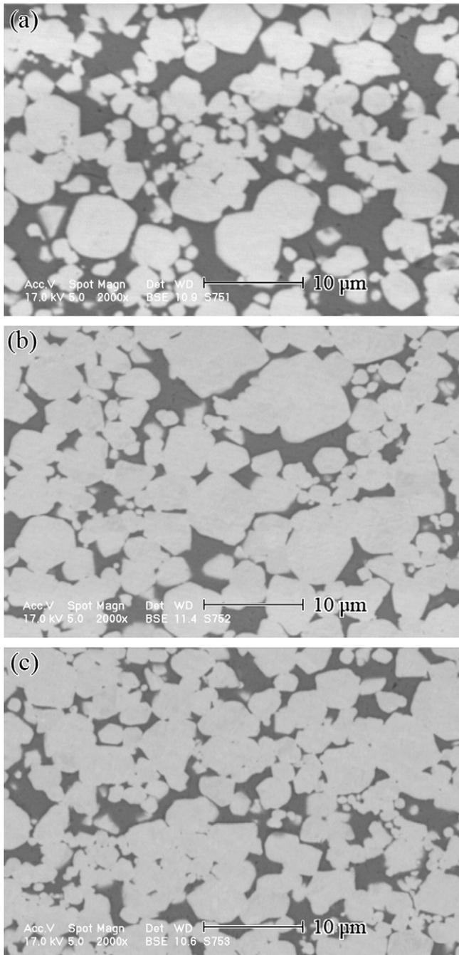
Fig. 3. Infiltrated green tungsten specimens without sintering compressed at: (a) 245 MPa, (b) 491 MPa and (c) 663 MPa.
