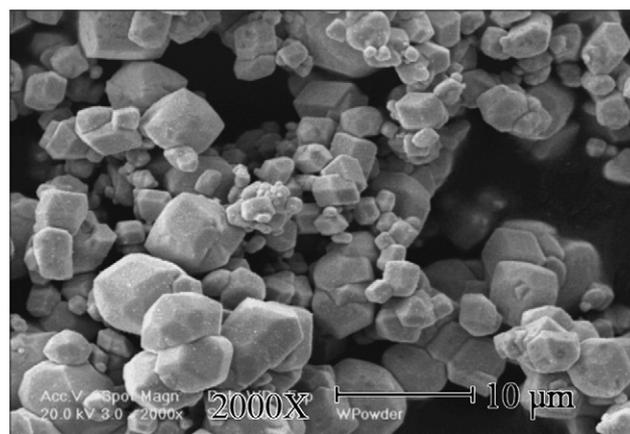
Fig. 1. Typical SEM micrograph of the initial tungsten powder.
