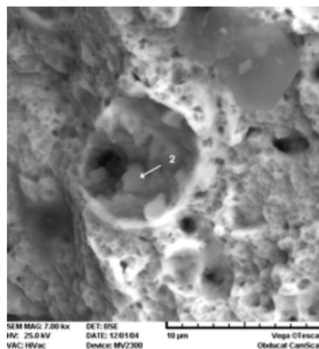
**Fig. 9.** Typical ductile dimples in the surfaces of fracture surface of casts 1 to 5.
