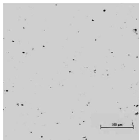
**Fig. 2.** Typical inclusions shapes, sizes and distribution in cast alloys.
