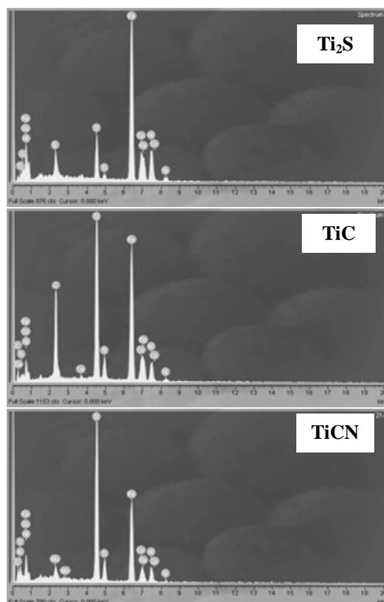
**Fig. 6.** Spectrographs showing typical analysis of inclusions shown in Fig. 6.
