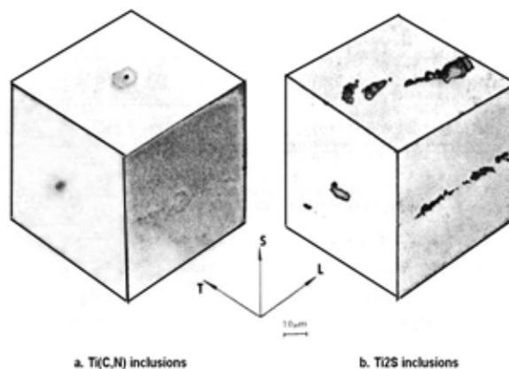
Fig. 1. Ti<sub>2</sub>S and Ti (C, N) inclusions shapes in high Ti high strength steel [10].
