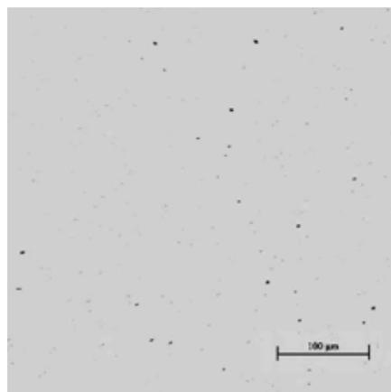
**Fig. 4.** Typical size, shape and distribution of inclusions in hot rolled bars.
