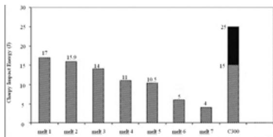
**Fig. 7.** Impact energy of aged specimens together with the impact energy of standard maraging C300 for comparison.
