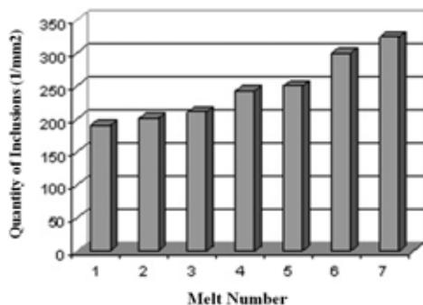
**Fig. 3.** Bar chart of inclusion number in various cast having different amount of Ti.
