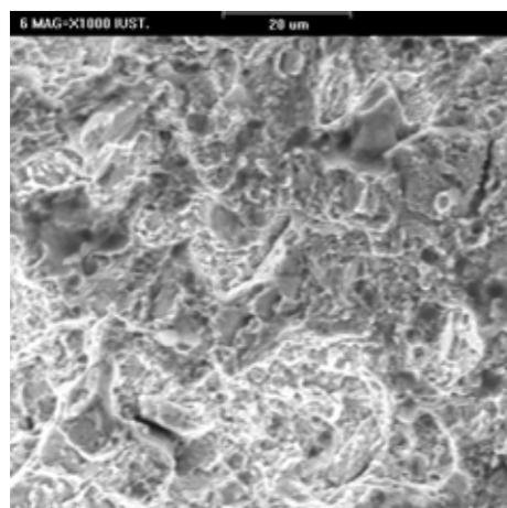
**Fig. 10.** Typical brittle fracture surfaces of casts 7.
