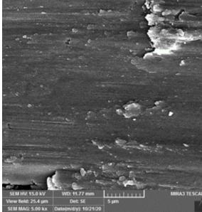
**Fig. 11.** shows an image of the reference sample surface after abrasion testing at a constant load of 300 g and a distance of 50 m, (a) before wear (b) after wear
