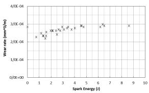
**Fig. 16.** Changes in wear rate with spark energy in wear under a load of 300 g force and a distance of 50 m.
