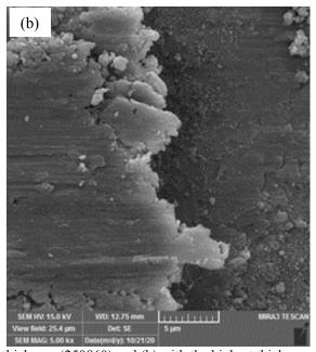
**Fig. 17.** Image of the sample surface (a) with the lowest thickness (250860) and (b) with the highest thickness (251170) after performing an abrasion test at a constant load of 300 g of force and a distance of 50 m.
