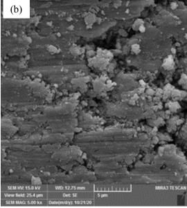
**Fig. 19.** Image of the sample surface (a) The sample with the lowest roughness (150550) and (b) The sample with the highest roughness (351170), after performing a wear test at a constant load of 300 g force and a distance of 50 meters.
