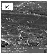
**Fig. 7.** The pin surface has been shown as follows: a) before the wear test, b) after 50 m wear on the reference sample at a constant load of 300 g, and c) after 50 m wear on the reference sample at a fixed load of 500 g.
