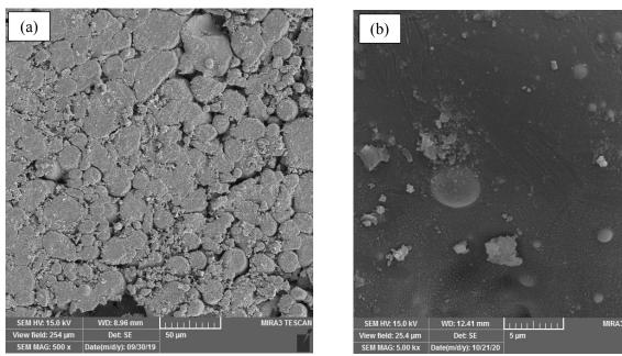
**Fig. 1.** SEM images of the (a) electrode microstructure and (b) the coated sample surface with the highest thickness (250860).
