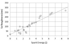
**Fig. 6.** Changes in surface roughness with spark energy
