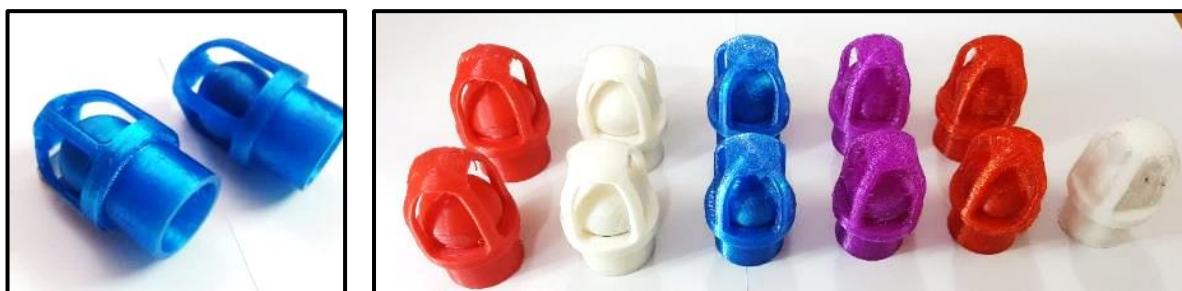
Fig. 5. The 3D printed artificial caged ball heart valves; PLA white; TPU transparent purple; TPE red; PETG blue
