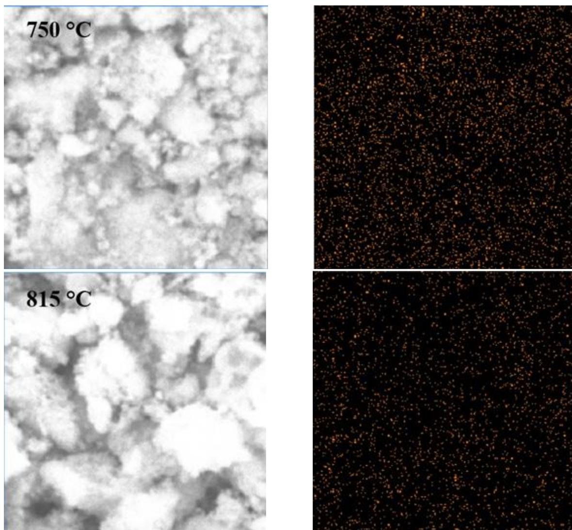
**Fig. 3.** Chlorine elemental mapping using EDS analysis at 750 and 815°C.
