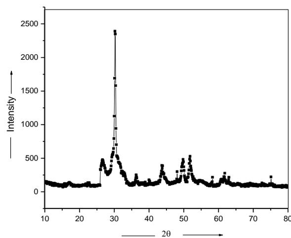
Fig. 2. XRD diffractogram of CdS thin film.
