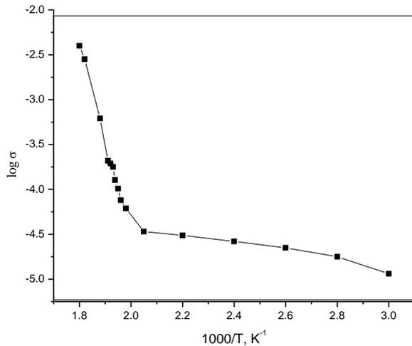
Fig. 3. Variation of electrical conductivity with working temperature for sample.
