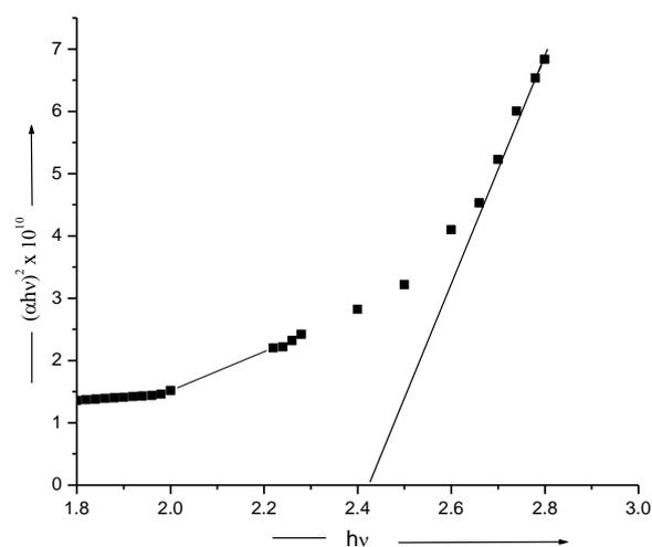
Fig. 1. A plot of  $(\alpha h\nu)^2$  vs  $h\nu$  typical as deposited CdS thin film.
