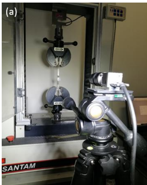
Fig. 4. a).Setup of the fracture toughness, b) before start test, C) end test
