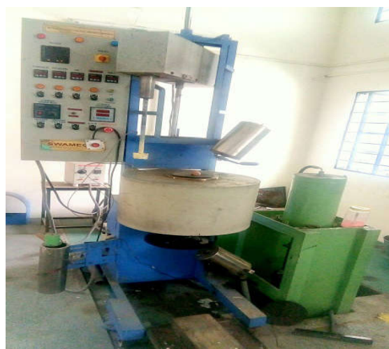
Fig. 1. Squeeze casting machine setup
