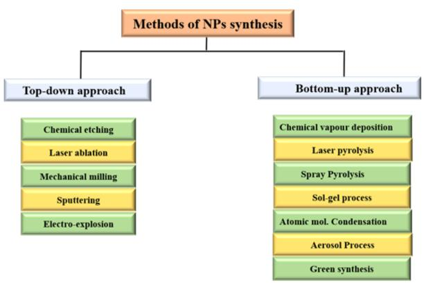
Fig. 2. Different methods of nanoparticles synthesis
