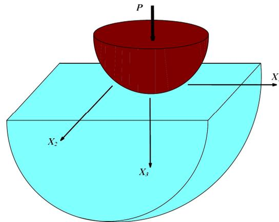
Fig. 1. The schematic geometry of orthotropic indentation
